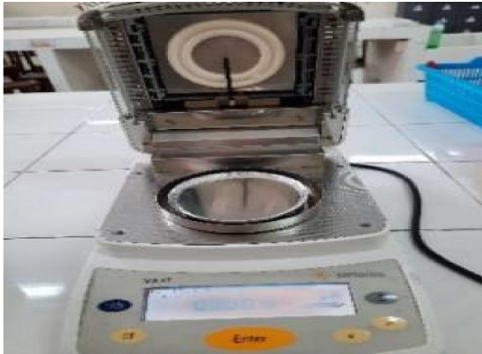
Gambar 2. Moisture Analyzer Type Sartorius MA-45
