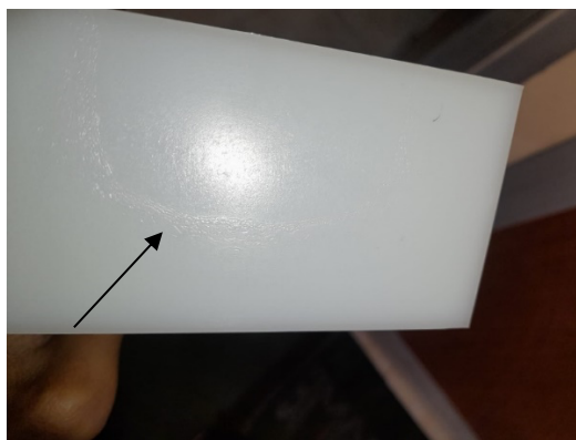
Gambar 3. Defect Weld line
